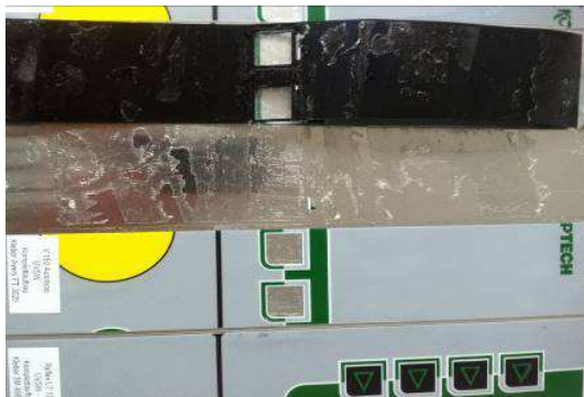
Adhesive splits itself (cohesive failure), no delamination of the colour structure
