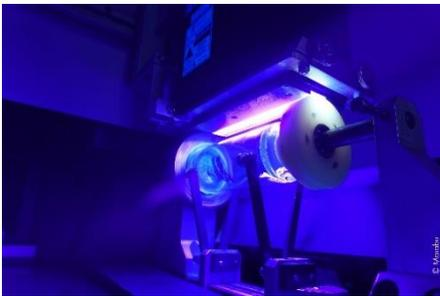
Industry players have come to value the many benefits of UV-LED curable products. Particularly for packaging, more and more manufacturers are equipping their printers with space-saving UV-LED lights. A key advantage over conventional halogen is that the UV-LED wavelengths are in the UV-A range. Consequently, they do not generate ozone emissions. The UV-LED unit comprises an array, i.e. an assembly of multiple individual LEDs. In the printing industry, wavelengths in the 385nm to 395nm range
