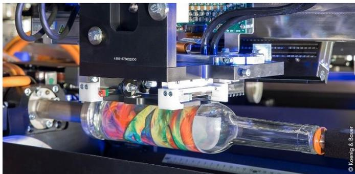
products of all kinds, from one-off items to large industrial-scale volumes – in conjunction with excellent results. Contours, for instance, are far sharper than with conventional embossing. The precise single pass application of multiple varnish layers is possible, producing extremely textured finishes. This is performed with printing systems from Koenig & Bauer's KAMMANN K15
